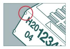
It also possesses four raised pips in the corners of the print face to protect the printed surface during dewaxing, while enabling the surface to be cleared of wax. The pips act to hold the print face off the surface of the heated wax trimmer but keep it close enough for the paraffin wax to melt in the usual way.
